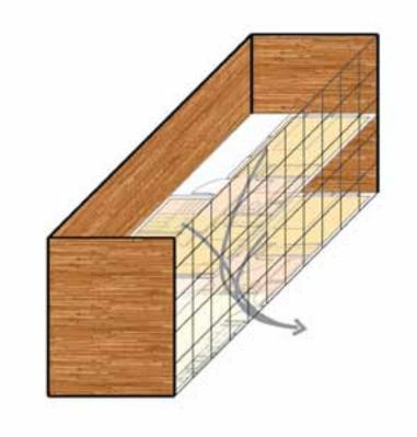
The three sided container is reiterated on the unit scale with three clapboard walls with a lighter panelized open wall. The units make use of modularity and off site construction. Their dimensions act as the building blocks of the cluster and site. Designed to optimize the 4'x8' panel and form a tight thermal envelope. The techtonics of manufactured housing is used for sustainability.
