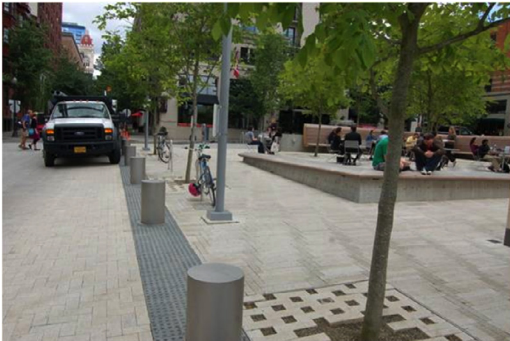
Figure 18: Curbless street demarcates pedestrian from vehicles by the use of bollards, location unknown.
