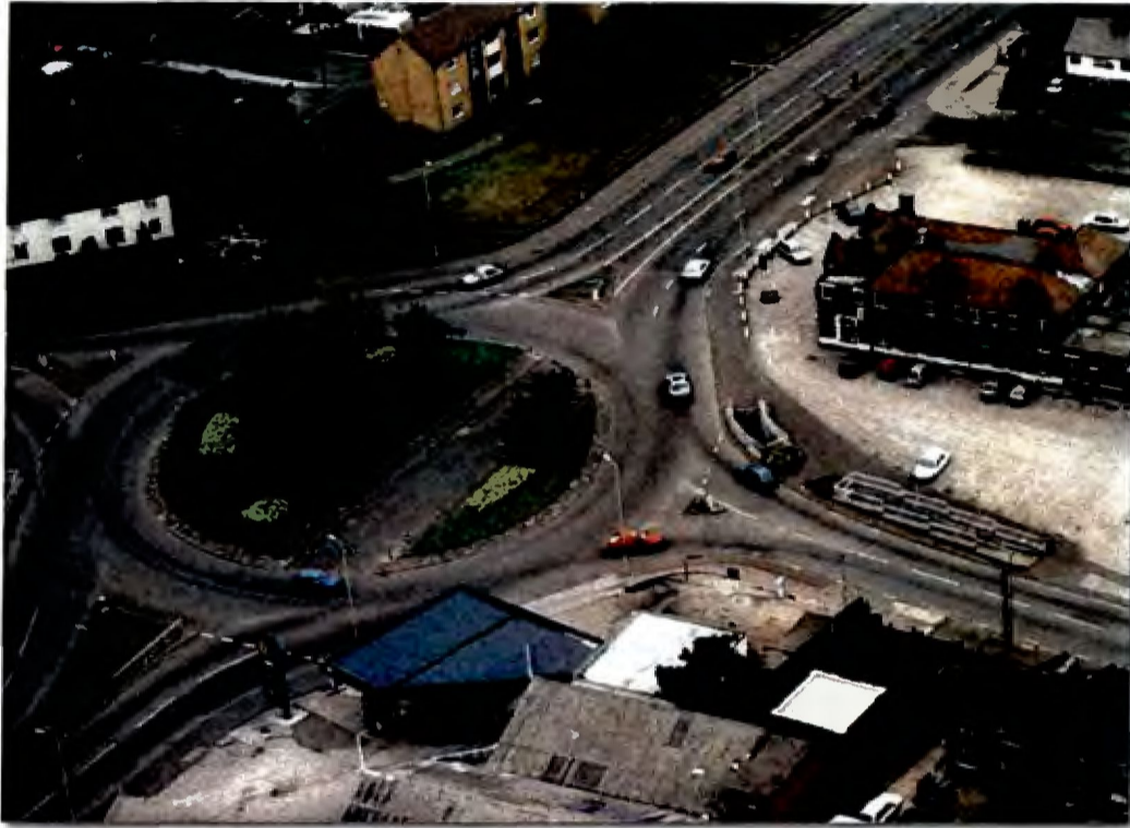
Exhibit 6-6 Example of a gated cut-through for heavy vehicles at a roundabout
