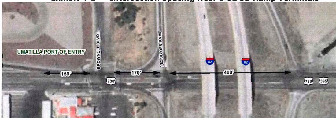
Exhibit 4-1 Intersection Spacing Near I-82 SB Ramp Terminals
