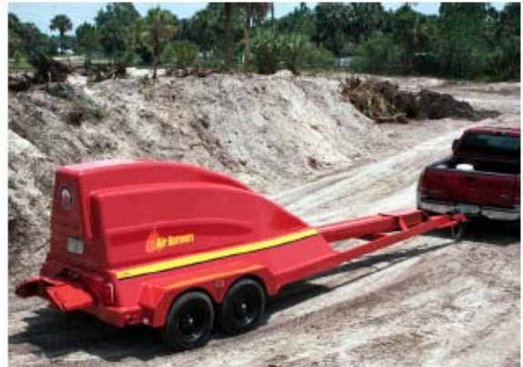
Figure 5—Trailer mounted trench burner system.
