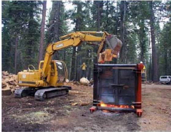
Figure 4—Loading fuel into ACD (full operation).
