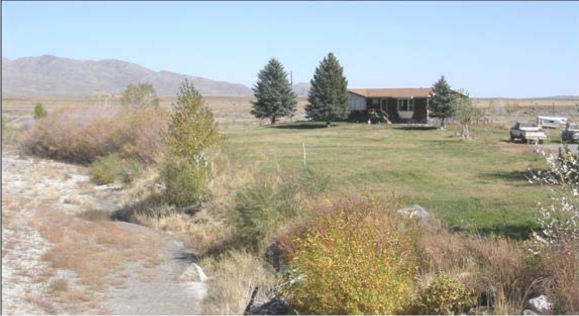
Figure 25. Single-family dwelling located along the Big Lost River This home 2 miles southwest of Butte City shows good defensible space, a metal roof, and landscaping back from structure.
