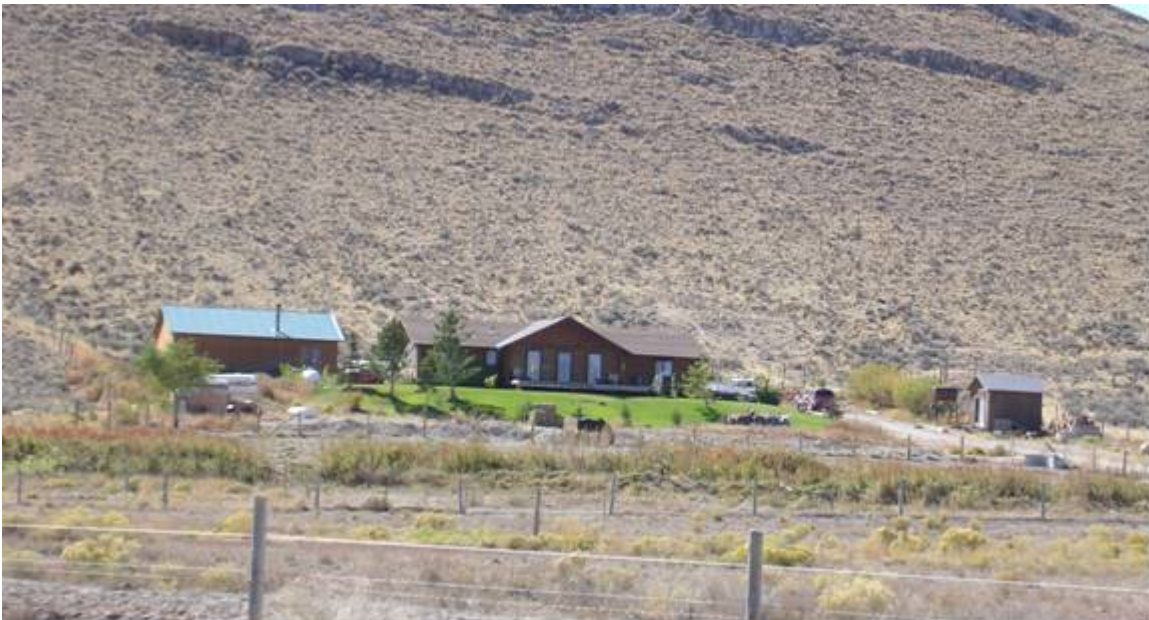
Figure 31. Single-family dwelling along the Little Lost River Valley Highway. This home is 1.5 miles northwest of Howe and shows good defensible space, metal roofs, and landscaping 30 feet beyond structures.
