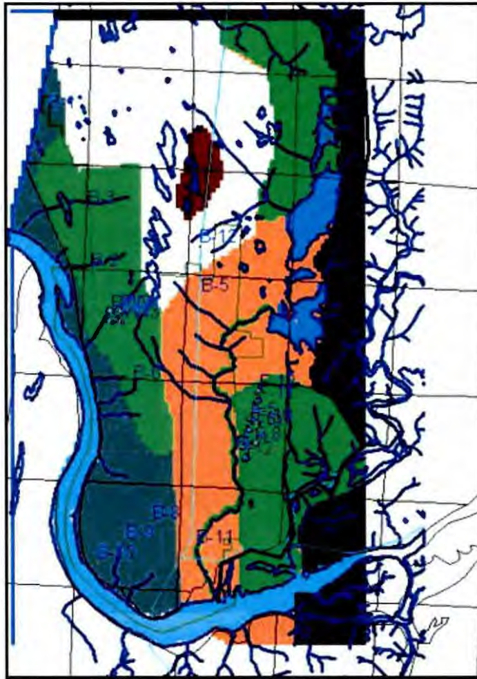
Figure 6. Variation of hydraulic conductivity within the sand aquifer. Colors represent the following K values (ft/day): green = 55, white = 35, orange = 18, gray = 15, brown = 5.
