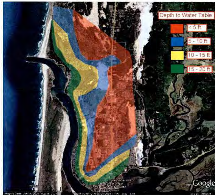
Figure 7. Approximate depth to the water table in the Florence Dunal Aquifer. This map is based on measurements taken at the monitoring wells in the City. Data reflected here were collected in April 2011, when the water table, coincident with rainfall, was high. Notice that the depth to the water table increases as one approaches the Siuslaw River Estuary.
