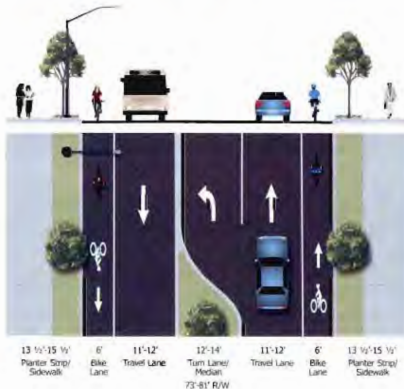
FIGURE 3-7. MINOR ARTERIAL CROSS-SECTION
