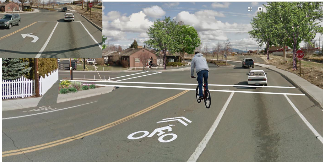
After: Turning lane with sharrow on Canal Blvd.
