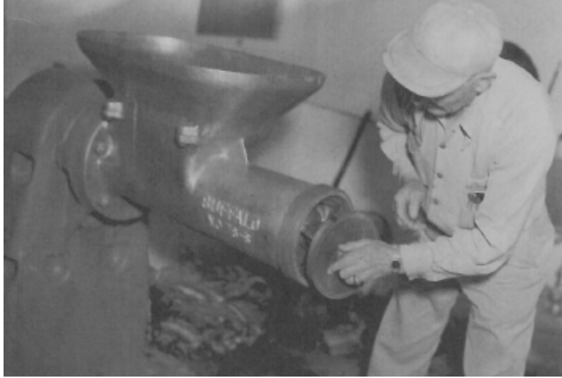
Figure 2.8. Meat grinder used in preparing feed for juvenile salmon, Oakridge Salmon Hatchery (Willamette Hatchery) c. 1955. Courtesy Oregon Historical Society Research Library, OrHi 3499, Lot 790, Box 14, Folder 17.
