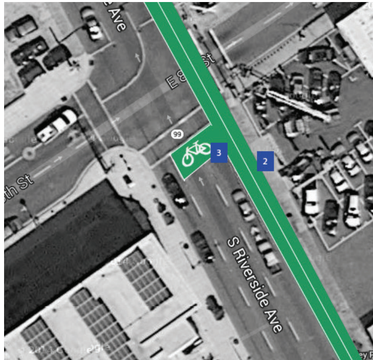
Figure 25: Aerial view of a bike box proposed for intersections on Riverside Avenue/ OR-99
