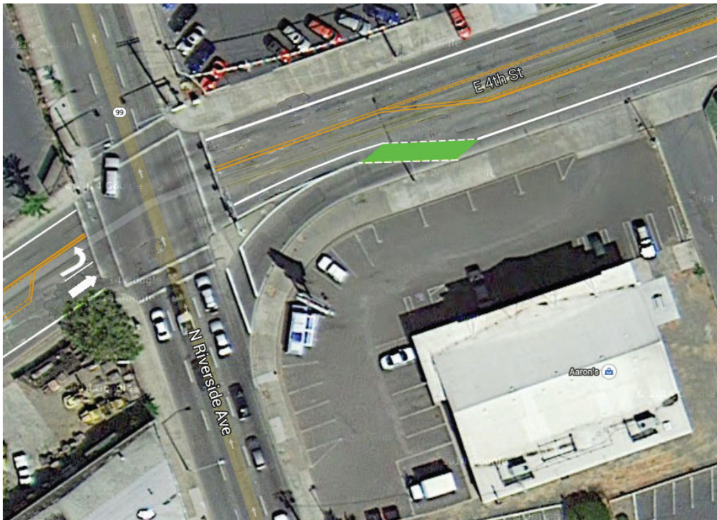
Figure 31: Vehicles turning right onto 4th Avenue from North Riverside Avenue pose a potential safety risk for cyclists.
