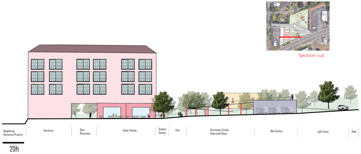
Figure 104: Section of the site from east to west. The market would have an open bottom floor to allow for permeable entrances and seating options.
