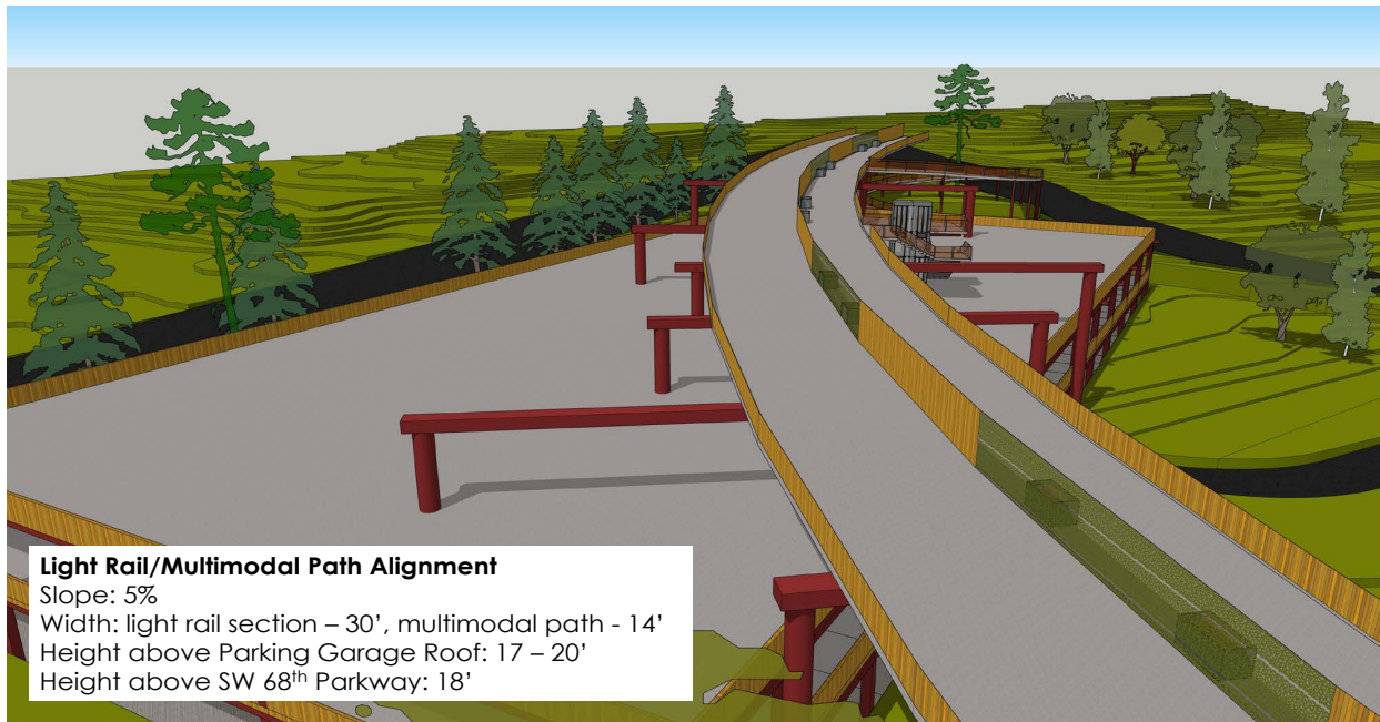
Figure 20: Perspective model of the garage in relation to the light rail line and multimodal path.
