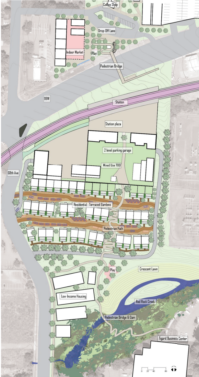
Figure: 65: Site plan with each zone’s 80-scale design and their relationship to the light rail and station.
