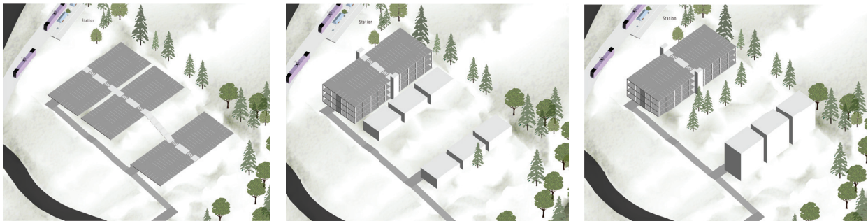
Figure 30: Traditional Park and Ride and development strategies. Option 1: a parking lot, option 2: a garage and development, and option 3: garage and development setback.
