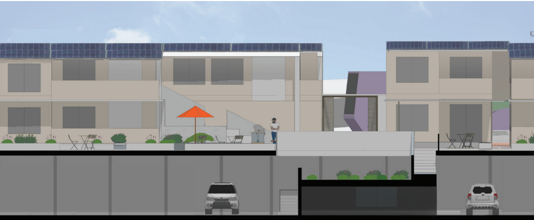
Figure 38: A section cut facing east visualizes the spatial relationship between the garage, corridor, and residential units.
