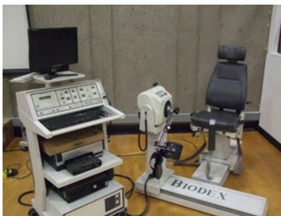
Figure 2: Biodex 3 dynamometer used to assess hip abductor strength
