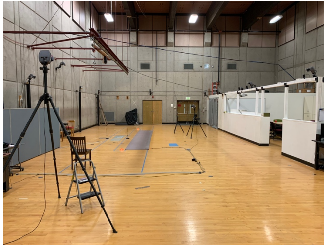
Figure 1 Flat, hardwood walkway for subjects to walk across, then to circle back to starting position. IR camera setup is also seen around the walkway.
