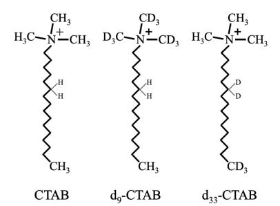
**Figure 3.1.** Chemical structure of fully hydrogenated CTAB, deuterated head group CTAB (d<sub>9</sub>-CTAB), and deuterated tail CTAB (d<sub>33</sub>-CTAB).
