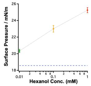
**Figure 4.1.** Surface pressure measurements for 0.1mM CTAB alone (blue dashed line) and when mixed with 0.01mM hexanol (green), 0.1mM hexanol (yellow), and 1mM hexanol (red).
