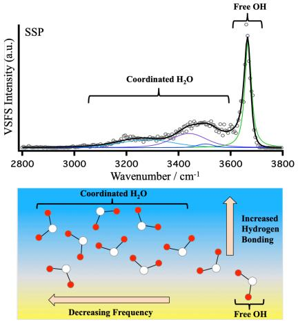
**Figure 2.4.** VSFS spectra (*ssp* polarization) of the neat  $CCl_4 - H_2O$  interface, with labeled Free-OH and coordinated water region. Below is a cartoon representation of the Free-OH residing in the oil phase with no hydrogen bonding, the companion mode, and more tetrahedrally bound water molecules.
