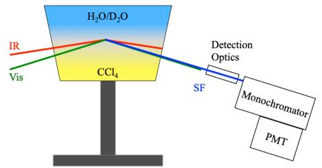
**Figure 2.3**. Schematic representation of the detection line, where incident visible and IR beams are overlapped at the  $CCl_4$  - aqueous interface to generate a third resultant sum frequency beam, which is detected by a monochromator and PMT.
