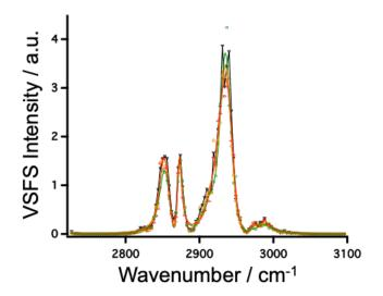
**Figure 4.3.** VSF spectra (*ssp* polarization) at the  $CCl_4 - D_2O$  interface of 0.1mM CTAB alone (black) and mixed with 0.01mM (green), 0.1mM (yellow), and 1mM (red) d<sub>14</sub>-hexanol. The  $I_{d+}/I_{r+}$  for each of the four spectra is calculated to be 0.9 ± 0.05. Solid lines are fits to the data.
