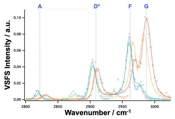
**Figure 3.5.** VSF spectra (*ssp* polarization) in the C-H region of 0.05mM (red), 0.1mM (yellow), 0.5mM (green) and 1.0mM (blue)  $d_{33}$ -CTAB at the CCl<sub>4</sub> – D<sub>2</sub>O interface. The solid lines are fits to the data.
