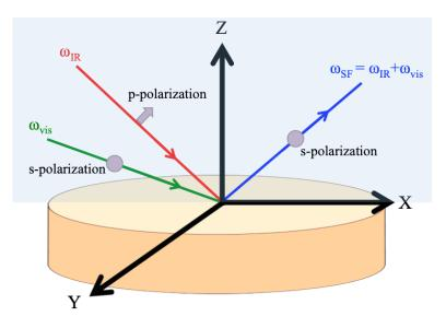
**Figure 2.1**. Schematic of the VSFS process at a  $C_{\infty}$  interface, in which the laser beams propagate in the xz-plane (shown in blue), and the interface lies in the xy-plane. Incident and resultant laser beams are depicted in the *ssp* polarization.
