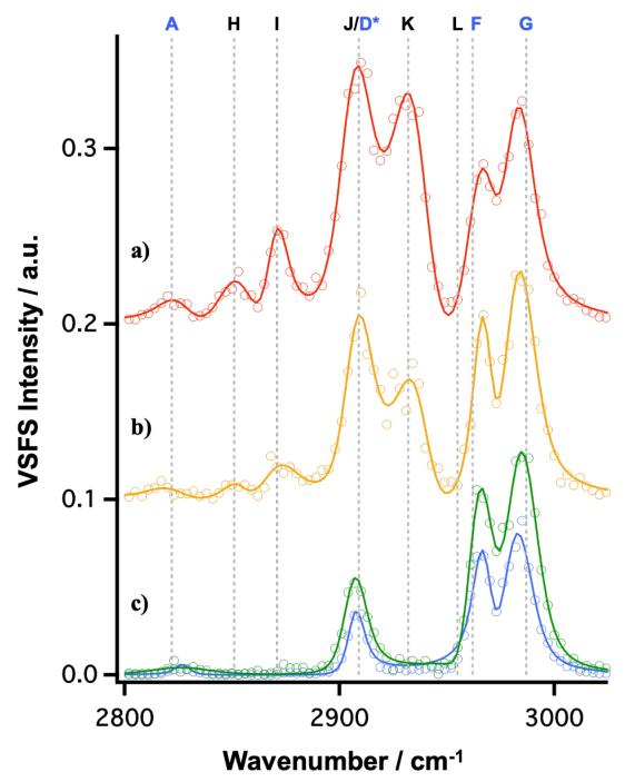
**Figure 4.2.** Offset VSFS spectra (*ssp* polarization) of the C-H region at the  $CCl_4 - D_2O$  interface of 0.1mM d<sub>33</sub>-CTAB (blue) alone and mixed with hydrogenated 0.01mM hexanol (green), 0.1mM hexanol (yellow), and 1mM hexanol (red). Solid lines are best fits to the data. Dashed grey vertical lines map fit peak locations to their denoted letter, with the blue and back letters corresponding to the head vibrations of CTAB and the tail vibrations of hexanol, respectively.
