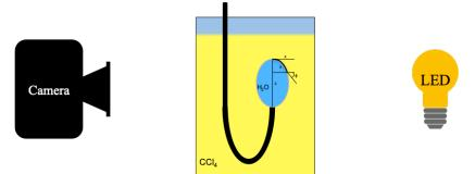
**Figure 2.5.** The pendant drop surface tensiometry set up used, showing camera, sample stage with hooked needle and backlight LED along with fitting parameters obtained from droplet.
