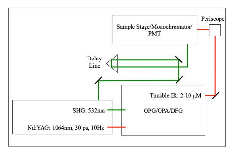
**Figure 2.2**. A simple schematic of the Ekspla laser system used to generate the visible (green lines) and infrared (red lines) beams need to generate VSFS.
