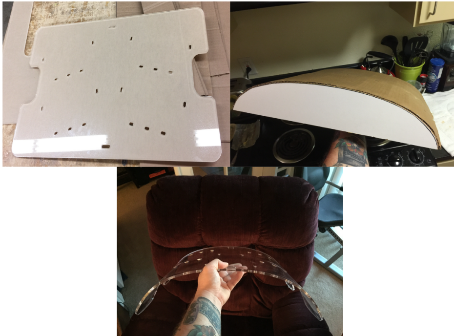
Figure 11: Final laser-cut acrylic piece (top left), wooden 'slumping' form (top right), final 'slumped' piece (bottom)
