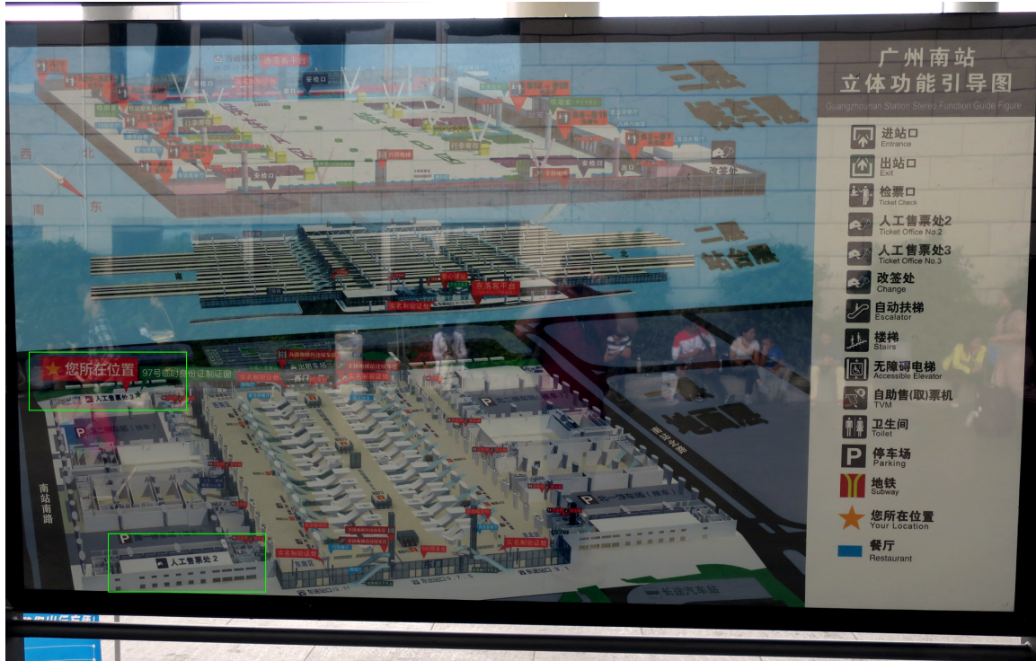
Figure 8.3. A map outside one of the ticket offices at Guangzhou South Station. Guangzhou South typifies the three layer “sandwich” design of new HSR stations, with a concourse open to the general public below the tracks and a shared waiting and boarding area above the tracks. Green boxes indicate the location of the ticket offices; that they are accessible from outside the station proper. Note that only ticket offices No. 2 and No. 3 are in service: the other two ticket offices, on the other end of the station, have been decommissioned.
