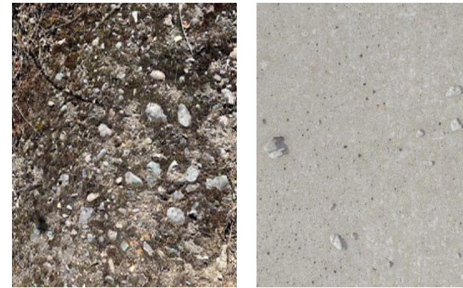
Figure 6.13: Contrast Between Original Dam Aggregate Concrete and Pumice-based. Left: Photo by author, March 2021. Right: From https://www.nemotile.com/verve-cement-pumice-12x24.html , accessed April 21, 2021
