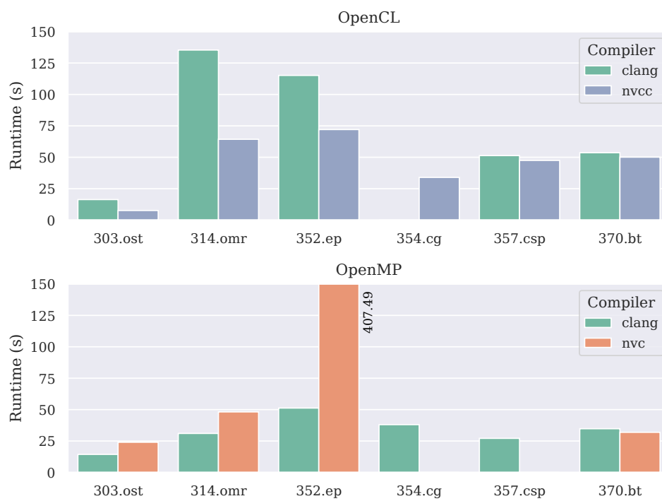
Figure 33. Runtime performance comparison of two OpenCL implementations and two OpenMP implementations (A100).
