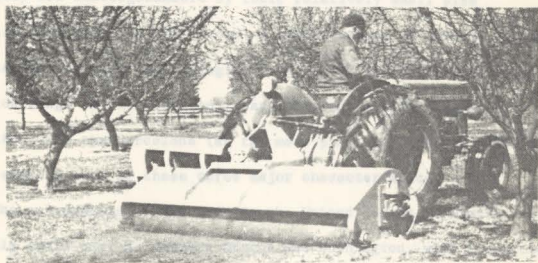
A flailing machine - a substitute for cultivating the orchard's grounds.
