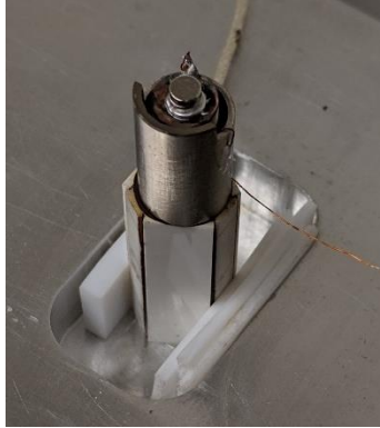
Figure 8.3. Fully assembled magnetic STM scanner assembly. NOTE: The current design uses 38 AWG coax cable for the tunneling current wire, and not the 34 AWG twisted pair visible in this picture.
