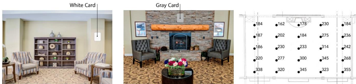
Figure 34. The location of white and gray cards within the experimental space and a 1.2 m horizontal grid of lux measurements
