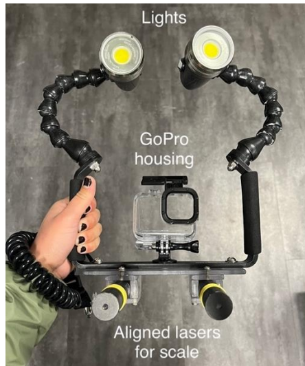
Figure 2. Camera rig used for video surveys. Equipped with lights, GoPro™, and aligned lasers. This system was modified from the rig originally described in Amsler et al. (in press).
