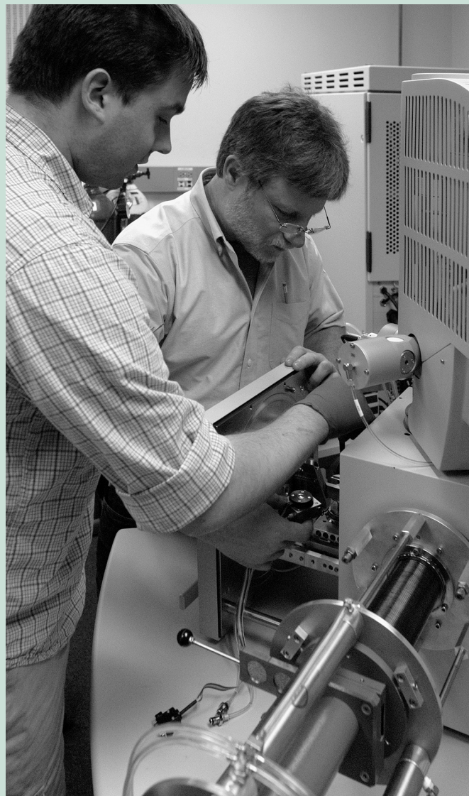
Michael Anderson (foreground) and John Donovan prepare to analyze a sample of sediment from 100 meters below the ocean floor using the Environmental Scanning Electron Microscope. The instrument is fitted with a custom-made cathode luminescence detector designed by Donovan and Kris Johnson of the UO machine shop, and is being used in a collaborative project with Pacific Northwest National Laboratories to measure the effects of global warming.
