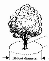
Figure 130-18. Measuring the Root Protection Zone
