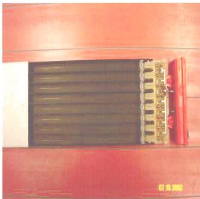
Fig. III.10: Top view of an LST module. The protective sleeve has been partly retracted for a better view.
