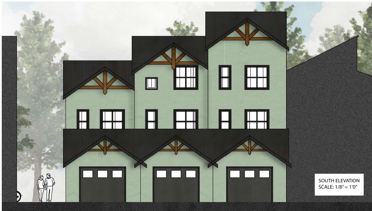
FIG. 20 Back elevation of cascading townhomes, showing parking strategy. Design Credit: Macy Moore
