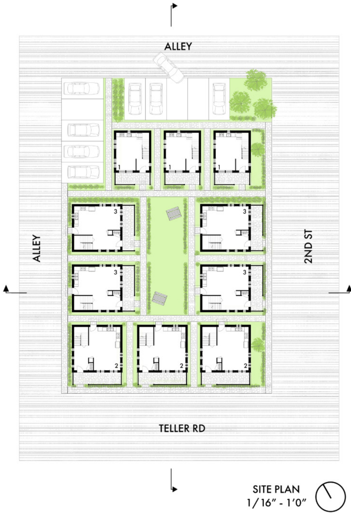
FIG. 34 Cottage Cluster site plan and first floor plans. Design Credit: Lily Maas
