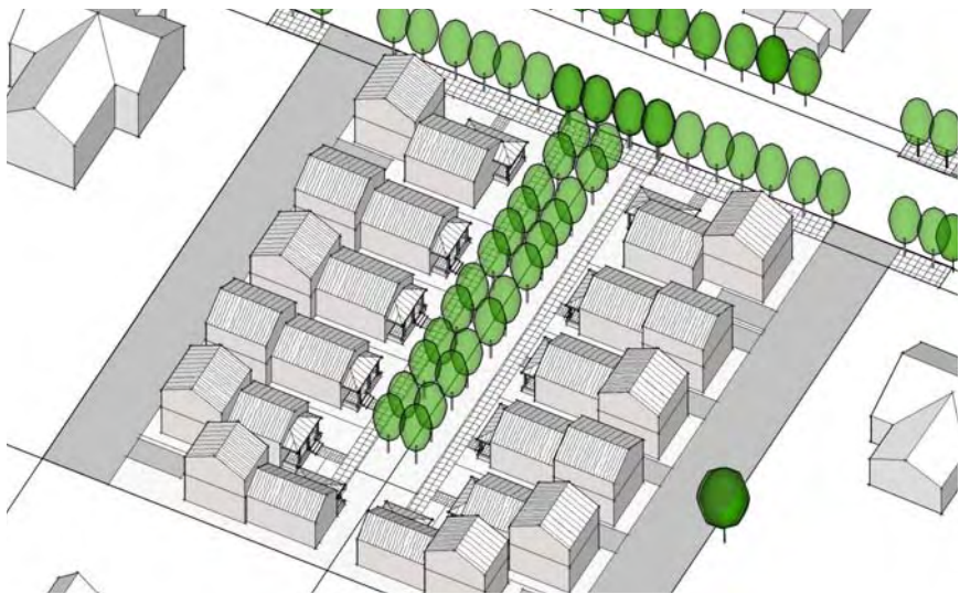
Without sprinklers (20'-wide accessway required)
