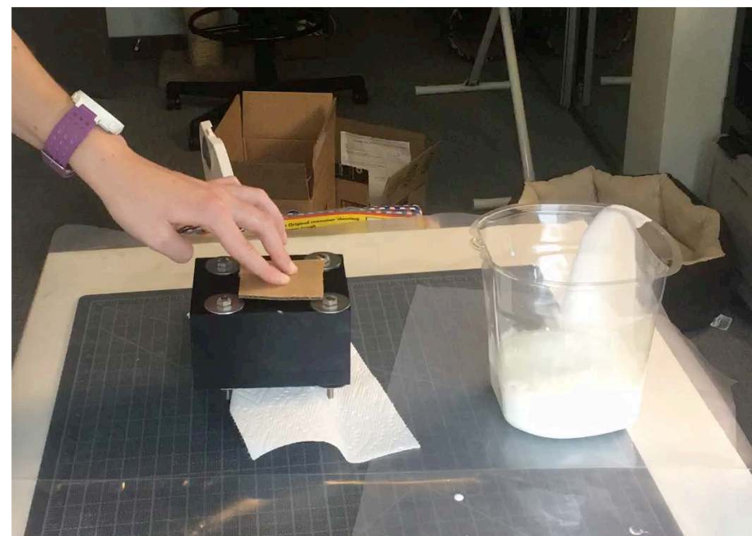
Testing out a 3D printed mold with Smooth-on casting
