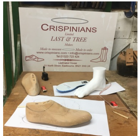
Fig. 17 The last was frequently compared to the outline and measurements to work towards the correct shape and size.
