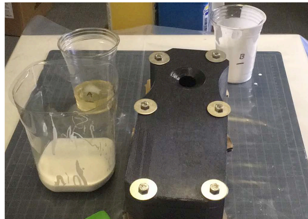
Casting works-like midsoles
