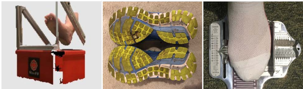
Fig. 14 3D foot scans were taken of the three women, Eleanor, Jessica, and Robin (right). Their shoes were also analyzed (center) and their feet were measured on a Brannock device (left).
