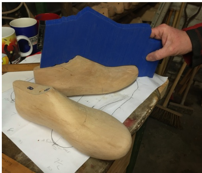
Fig. 18 A tool used to match curvature from one last to the other.
