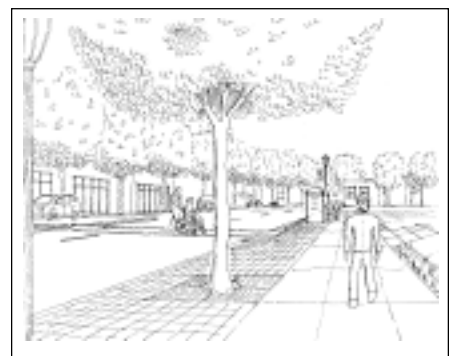
The sidewalk and furnishing zone treatment for the districts includes scored concrete sidewalks and permeable paver furnishing zones to provide district identity and stormwater management.
