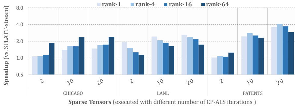
Figure 4.8. The performance of spCP-stream algorithm using ALTO-stream (without DTS) compared to the state-of-the-art SPLATT-stream across different factorization ranks (or tensor components).
