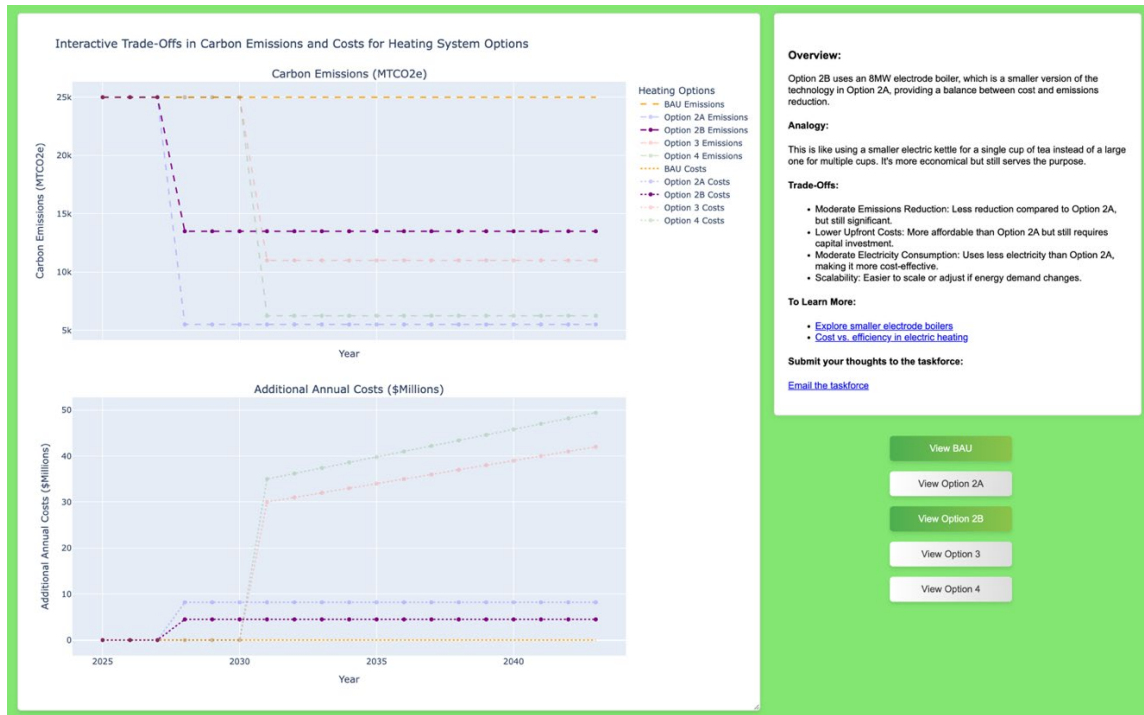
Figure 12: Dashboard Screenshot: Option 2B (8MW Electrode Boiler) button selected
