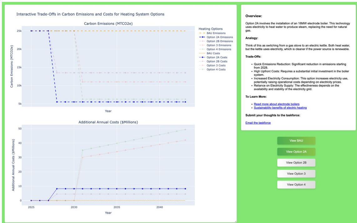
Figure 11: Dashboard Screenshot: Option 2A (18MW Electrode Boiler) button selected
