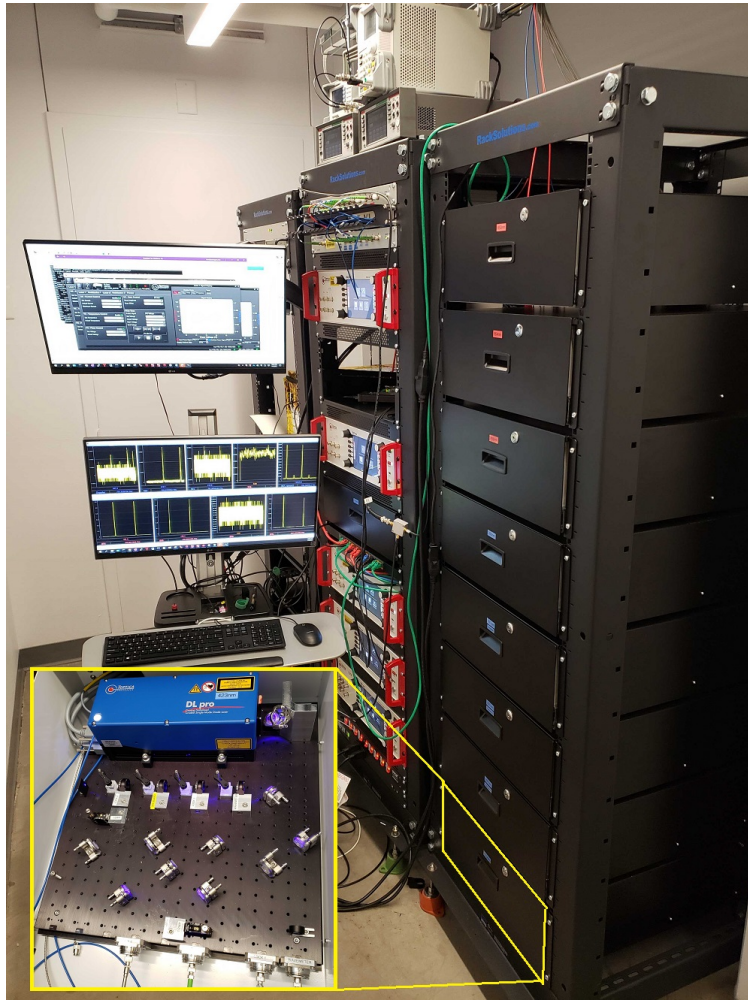
Figure 2.10. Photograph of our laser rack, showing the drawers containing laser breadboards as well as an additional rack for housing laser controllers and a third for the wavemeter and OSA board. Inset shows a sample laser breadboard mounted in a drawer.
