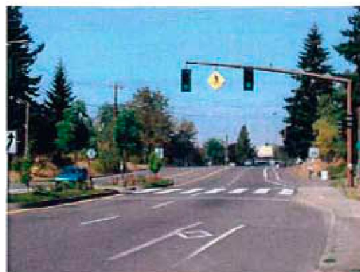
Figure 5-33: Type 3 crossing treatment.
