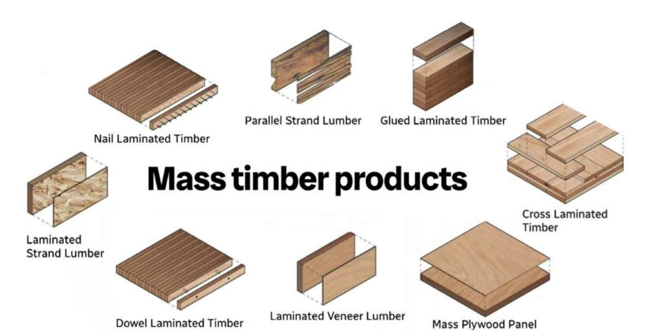
Types of Mass Timber Products Source: Mass Timber Institute, University of Toronto
