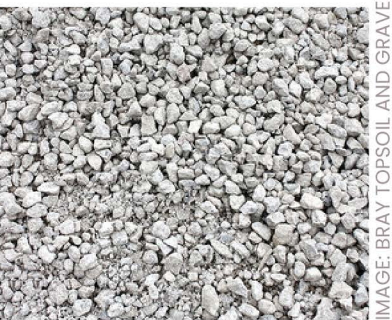
Crushed concrete aggregate
