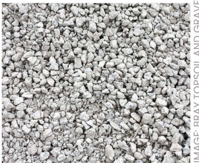
Crushed concrete aggregate
