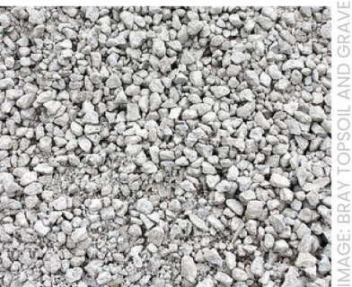
Crushed concrete aggregate
