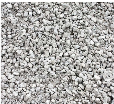
Crushed concrete aggregate
