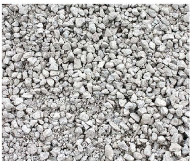
Crushed concrete aggregate
