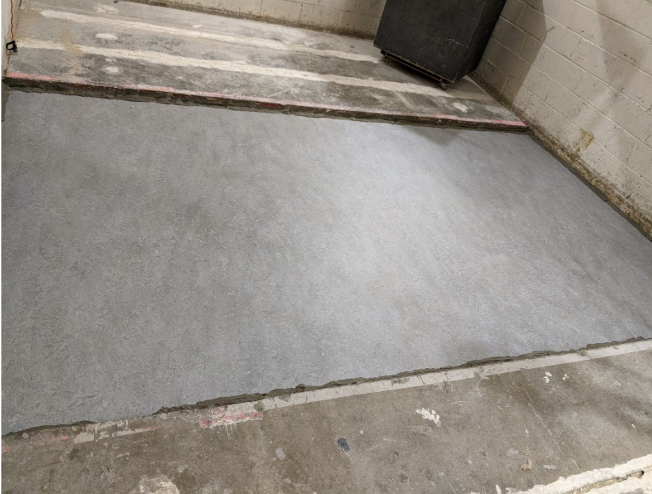
Figure 1 – Specimen mounted in test aperture, as viewed from source room
