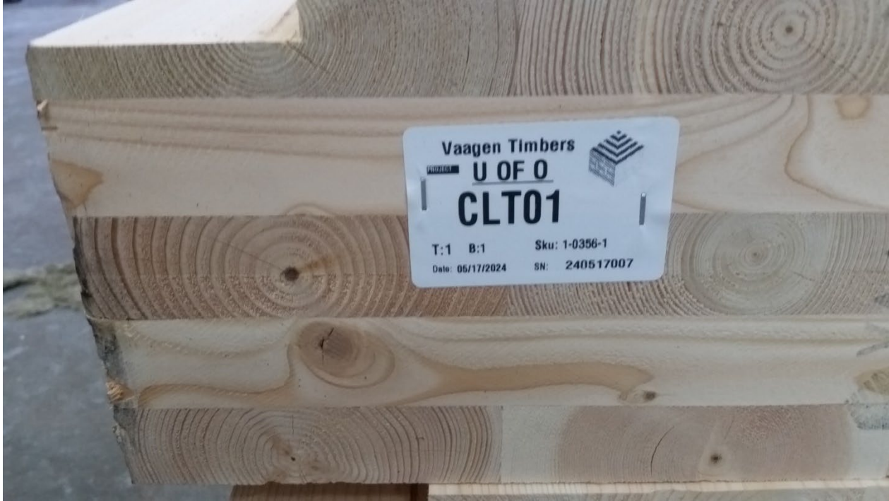
Figure 3 - CLT (1 of 2) prior to installation
