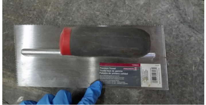
Figure 14 - Trowel used for installation of adhesive
