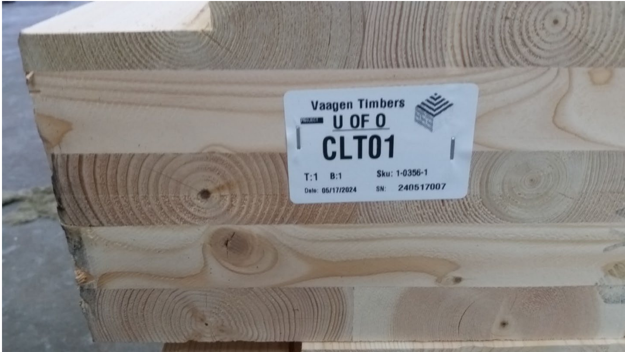
Figure 3 – CLT (1 of 2) prior to installation
