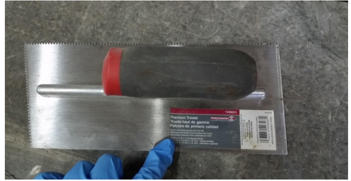
Figure 13 - Trowel used for installation of adhesive
