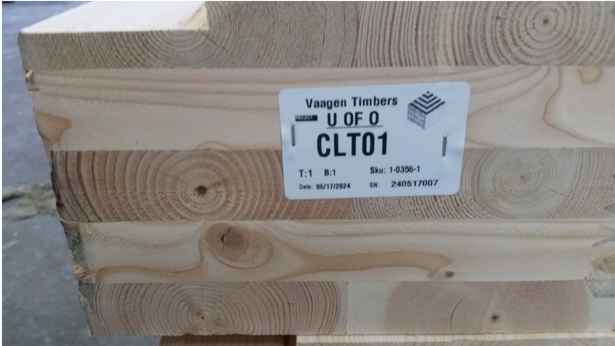
Figure 3 - CLT (1 of 2) prior to installation
