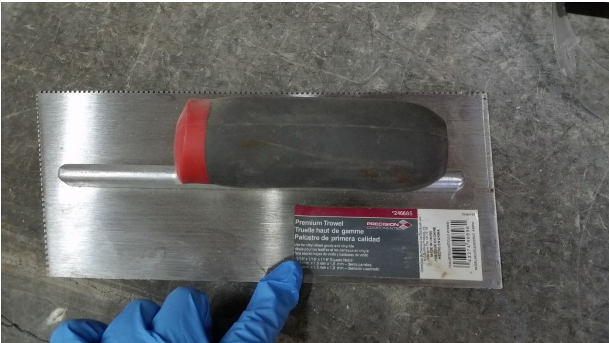
Figure 14 – Trowel used for installation of adhesive
