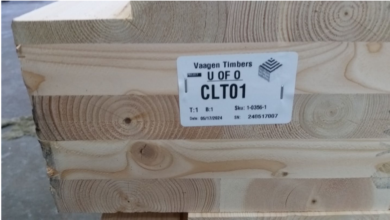
Figure 3 - CLT (1 of 2) prior to installation
