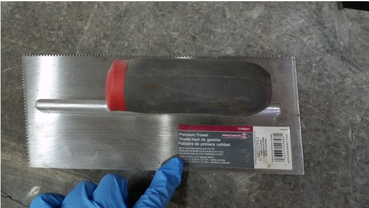
Figure 14 – Trowel used for installation of adhesive
