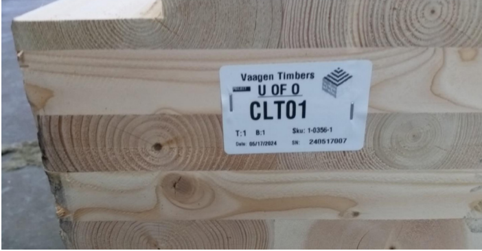
Figure 3 - CLT (1 of 2) prior to installation
