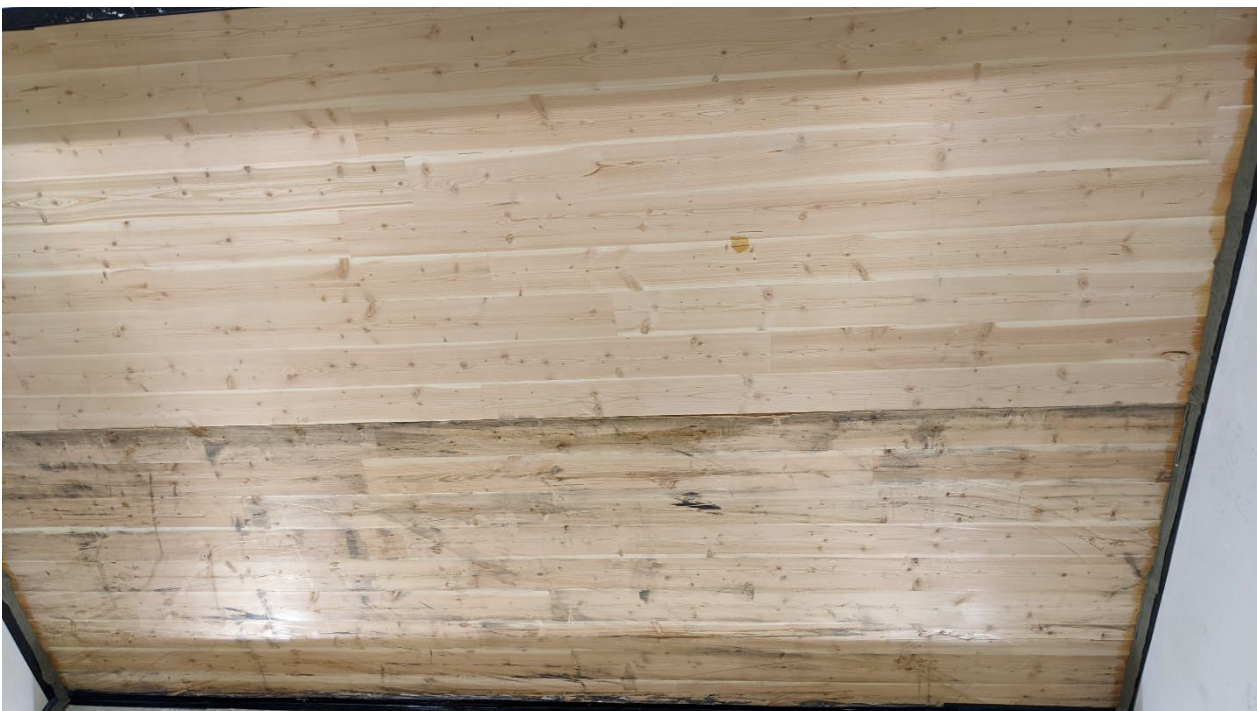
Figure 2 – Specimen mounted in test aperture, as viewed from receive room
