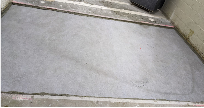
Figure 1 - Specimen mounted in test aperture, as viewed from source room
