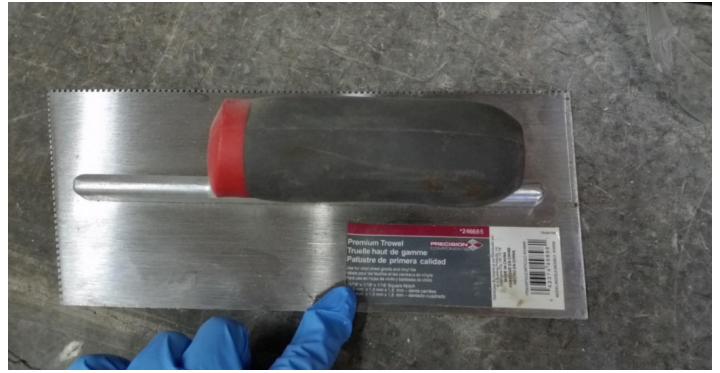
Figure 14 - Trowel used for installation of adhesive
