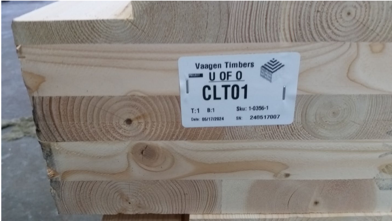
Figure 3 – CLT (1 of 2) prior to installation
