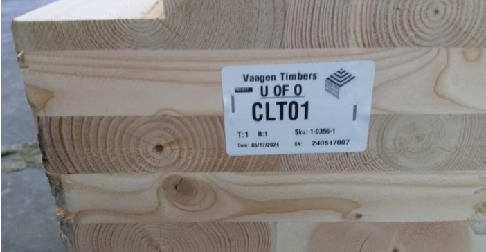
Figure 3 - CLT (1 of 2) prior to installation
