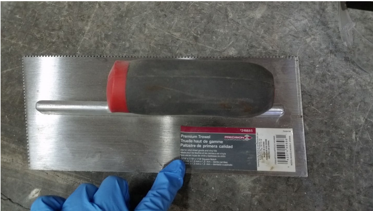
Figure 12 - Trowel used for installation of adhesive
