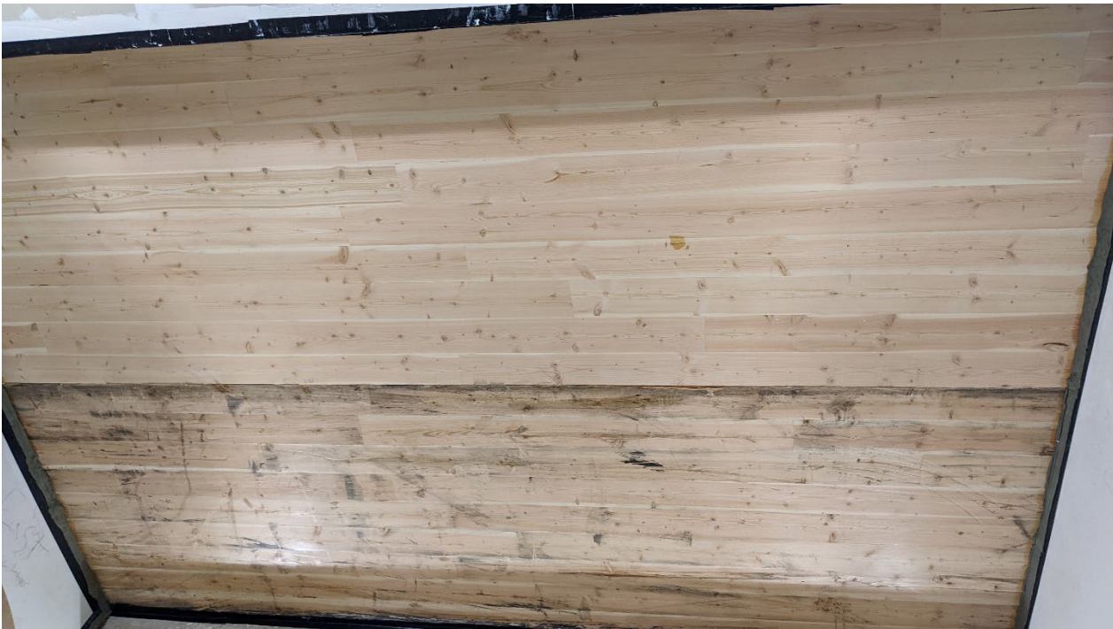
Figure 2 – Specimen mounted in test chamber, as viewed from receive room
