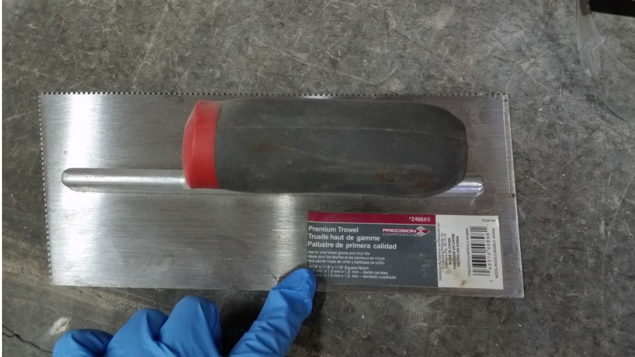
Figure 13 - Trowel used for installation of adhesive
