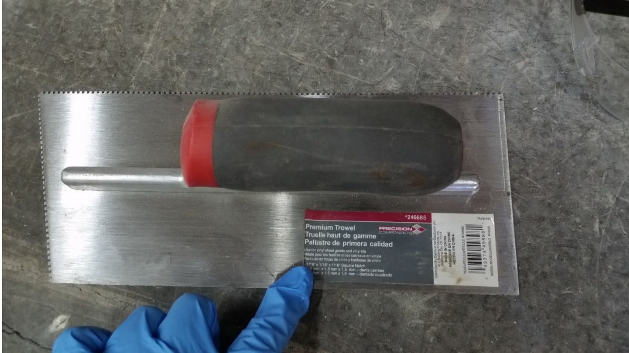
Figure 13 – Trowel used for installation of adhesive
