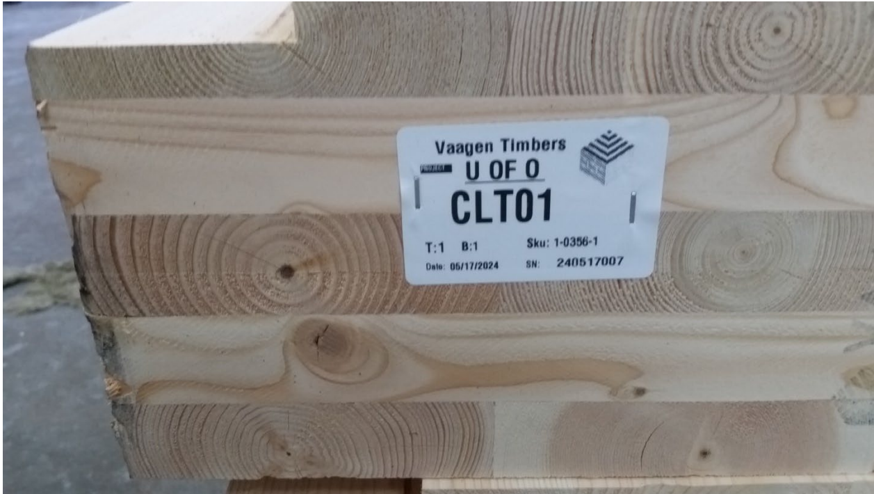
Figure 3 – CLT (1 of 2) prior to installation
