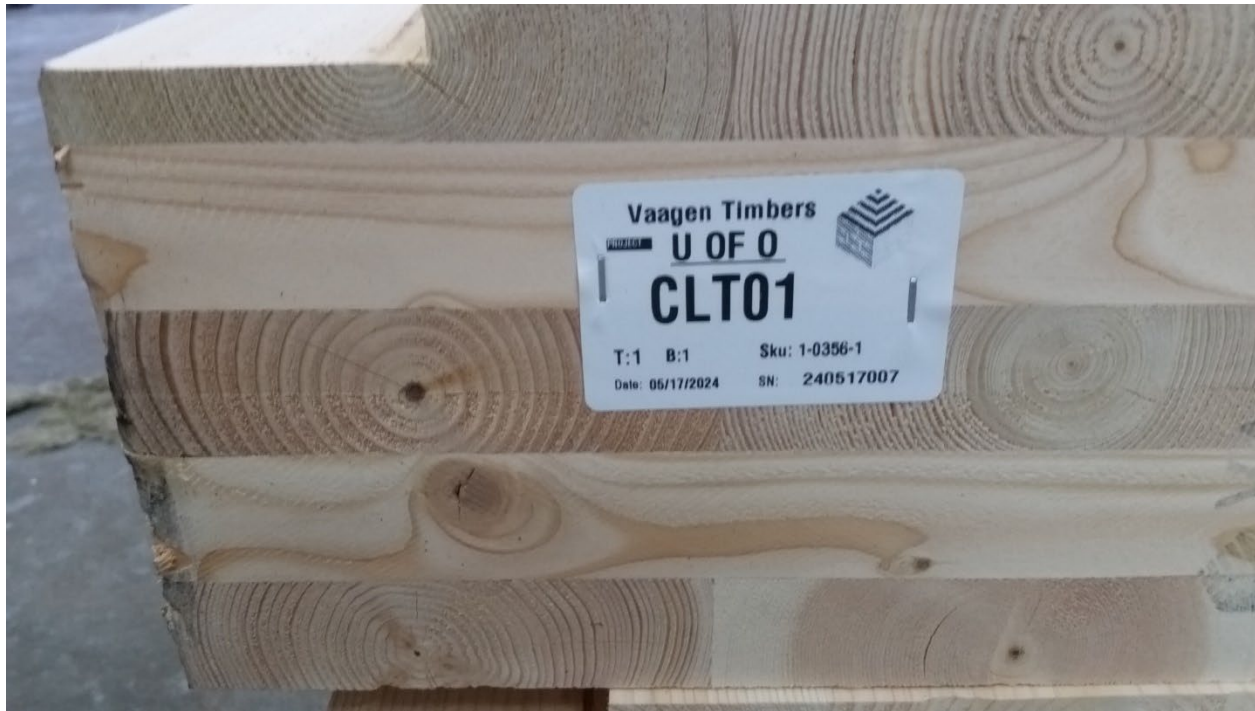
Figure 3 - CLT (1 of 2) prior to installation
