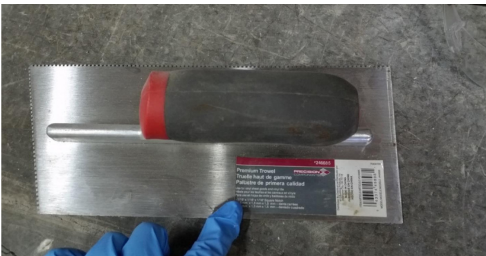
Figure 12 - Trowel used for installation of adhesive
