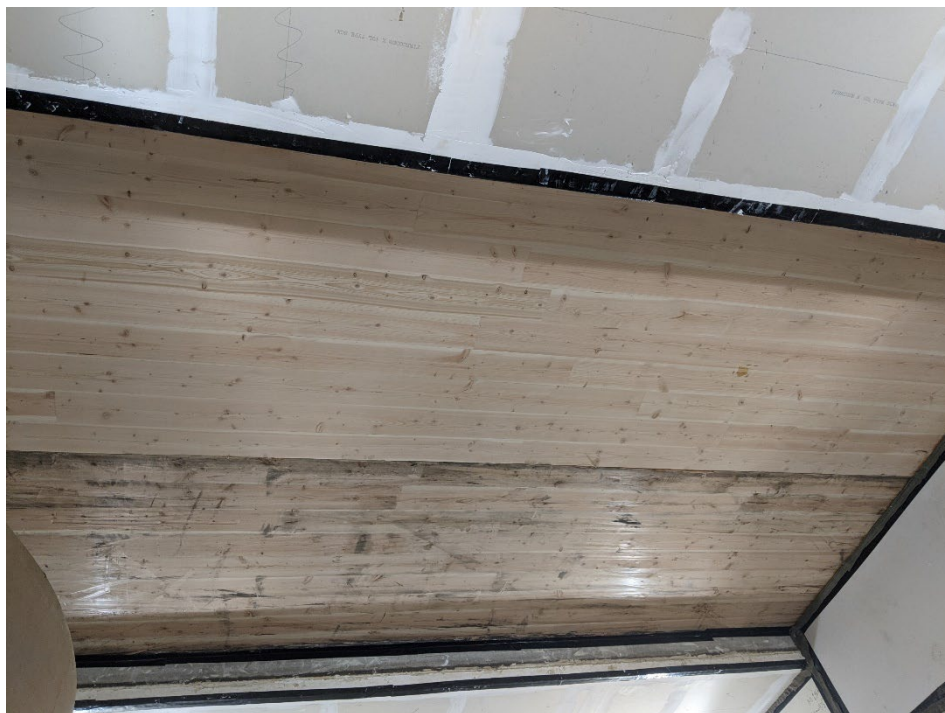
Figure 2 – Specimen mounted in test aperture, as viewed from receive room
