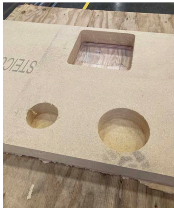
Images (clockwise from upper left): panel system over existing T1-11 wall, reflected to show inboard insulation and HVAC space, outboard insulation and ventilated cavity, flashings; panel foundation structural connections for seismic panel; rigid wood fiber insulation adhered to MPP and milled using CNC as a test case; fit of MPP panel window milled opening to existing LWF rough opening before application of interior finish.
