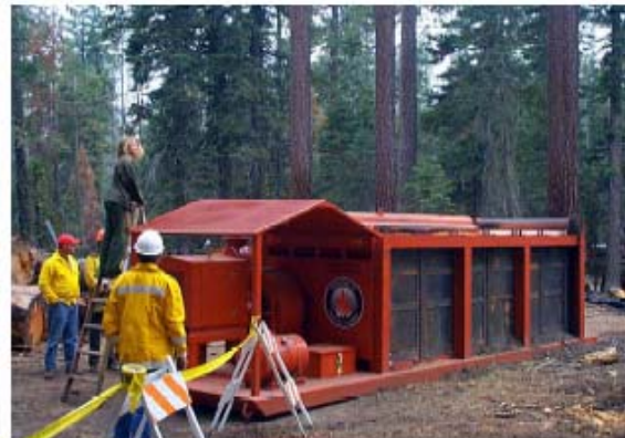
Figure 3—Skid mounted ACD in full operation (no visible smoke).
