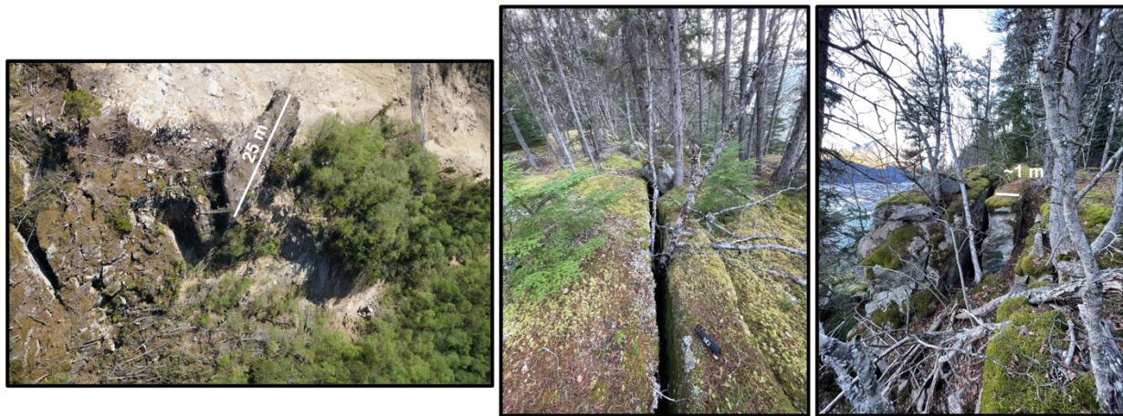
Figure 2: Rock slopes on the east side of Skagway valley with tension cracks and tall slabs of rock, consistent with the block toppling mode of failure.
