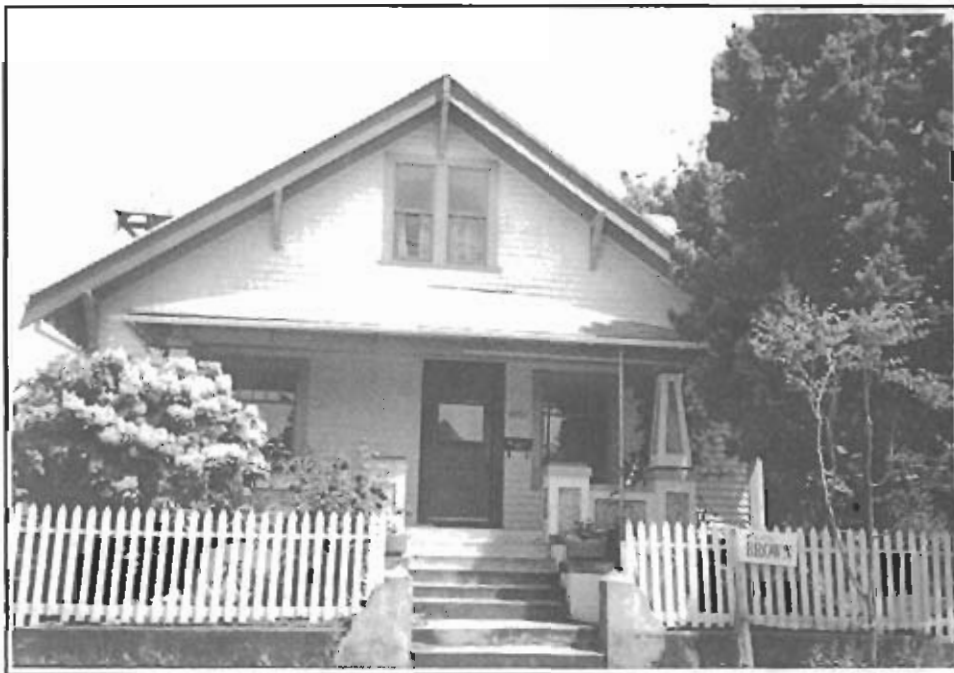
The strategically situated windows, dormers and porches of these homes encourage guardianship of the street space and heighten proprietary attitudes.
