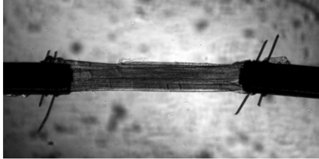
Figure 20. An image of a bundle of fibers with intact ECM mounted between a force transducer (left) and length motor (right).
