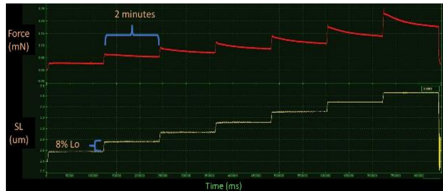
Figure 10. An annotated force and sarcomere length trace generated by the passive stiffness protocol. Each stretch step elongates the sample by 8% of initial length and holds this length for 2 minutes. At the end of the protocol, the sample is returned to initial length. The resulting trace is generally similar in fibers and fiber bundles.
