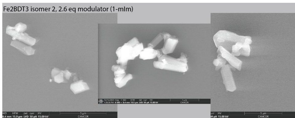
Figure 46. SEM images of \text{Fe}_2(\text{BDT})_3 with 2.6 eq 1-mlm modulator
