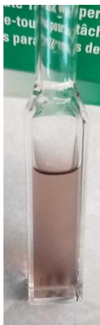
Figure 61. Photo of 18 nm MIL-125 in acetonitrile with decamethyl ferrocenium tetrafluoroborate in solution after being photodoped.
