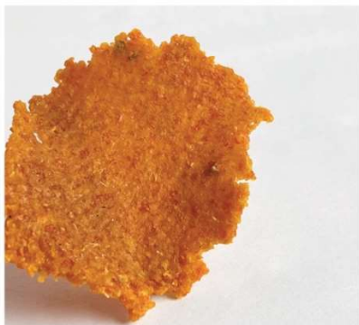
Experiment Number: 03 Ingredients: 5% Glycerin 57% Water 5% Agar 33% Blended orange peel Process: Cooked and poured Maya Merrill
