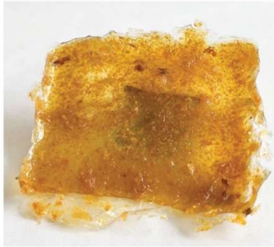
Experiment Number: 07 Ingredients: 5% Glycerin 70% Water 10% Gelatine 15% Blended orange peel Process: Cooked and poured Maya Merrill
