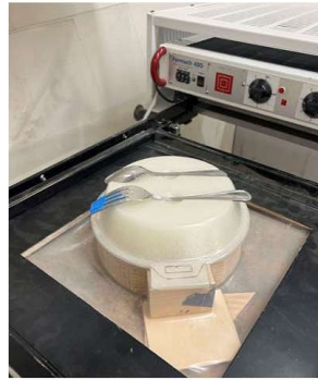
3. Vacuum form recycled PET plastic sheet around mold. 4. Press in silverware while plastic is hot.
