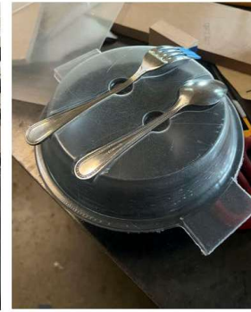
5. Cut around vacuum form after cooled. Trim excess PET, cut tabs with 1"x.25" holes and sand edges.
