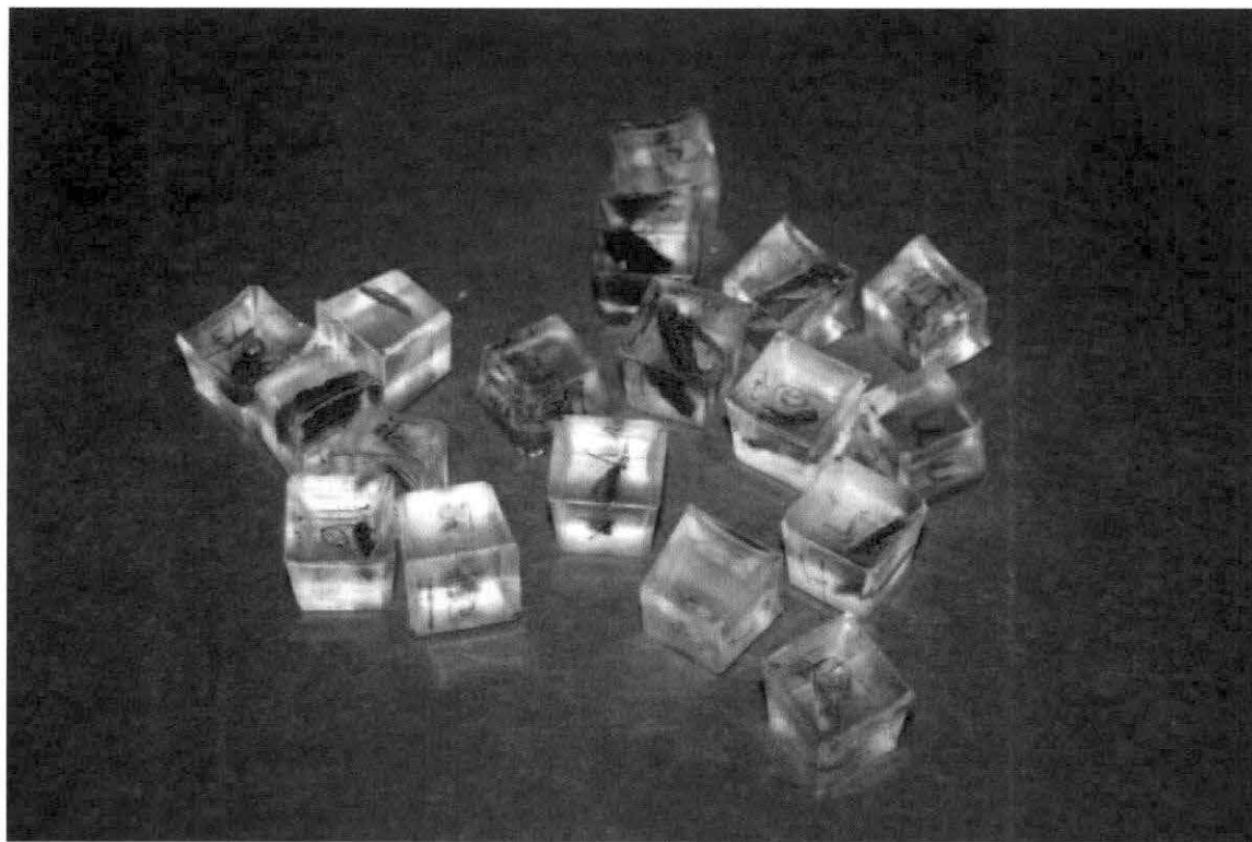
Fig. V-2. Photo of paint samples from HS-11 fixed in cast resin before sawing and color analysis.
