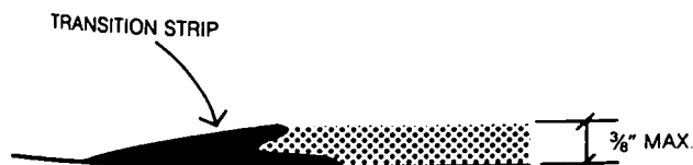
Figure 14.3 Flooring transition strip. Source: Department of Health and Human Services, Office of Facilities Engineering.
