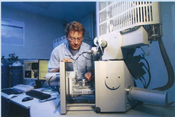
The Quanta 200 FEG, a scanning electron microscope, with a sample being set up for analysis.
