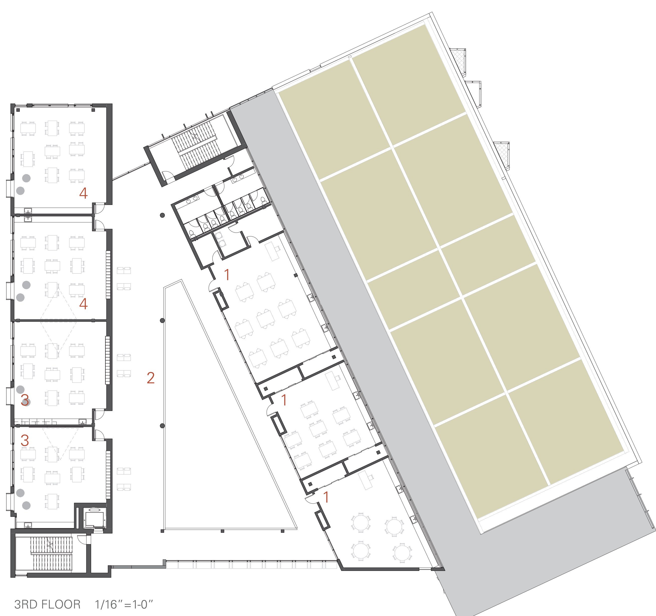
3RD FLOOR 1/16"=1'-0" 1. Art Rooms 2. Collaboration Space 3. Third Grade Classrooms 4. Fourth Grade Classrooms
