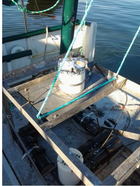
Figure 7. Sontek ADCP deployed by SSNERR 8 km up-estuary. Moored at 9 m depth.
