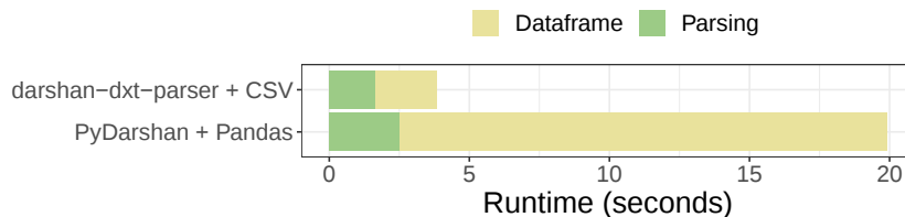
Figure 12. Comparison of methods to extract and combine the I/O behavior metrics from Darshan DXT traces required to pinpoint I/O issues and generate visualizations.
